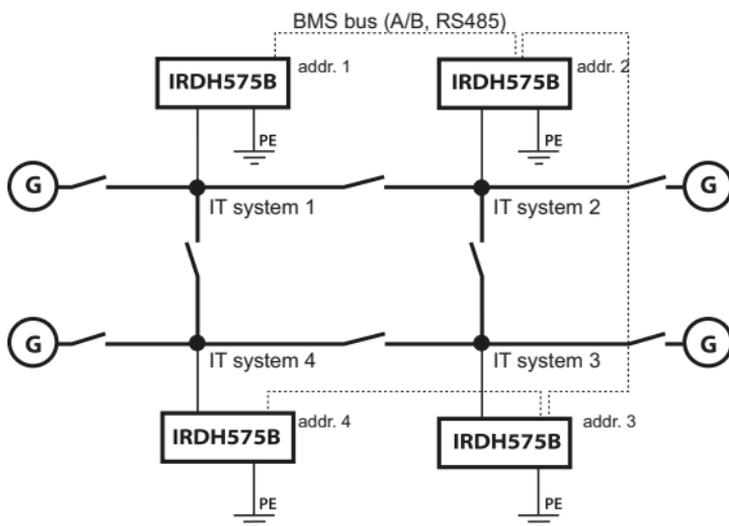
This has the advantage that no auxiliary contacts of a coupling switch are required. Furthermore, this solution is recommended for IT systems coupled via capacitances or diodes.
