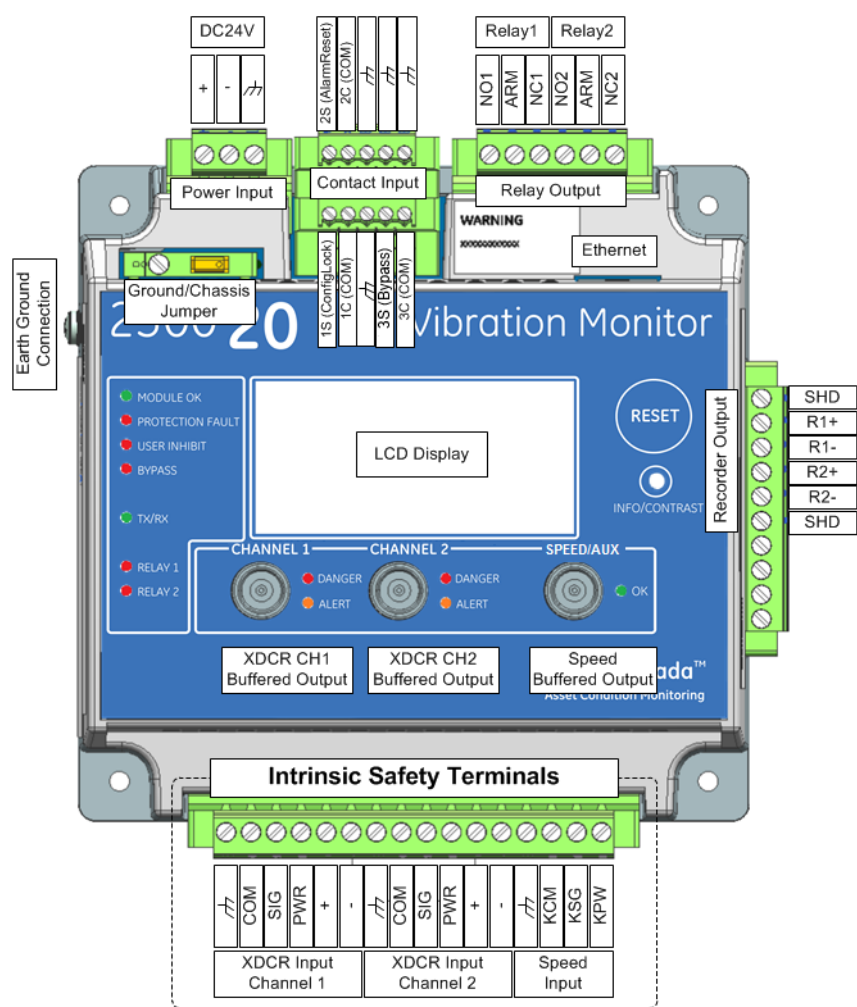
2300/20 Wiring Diagram
