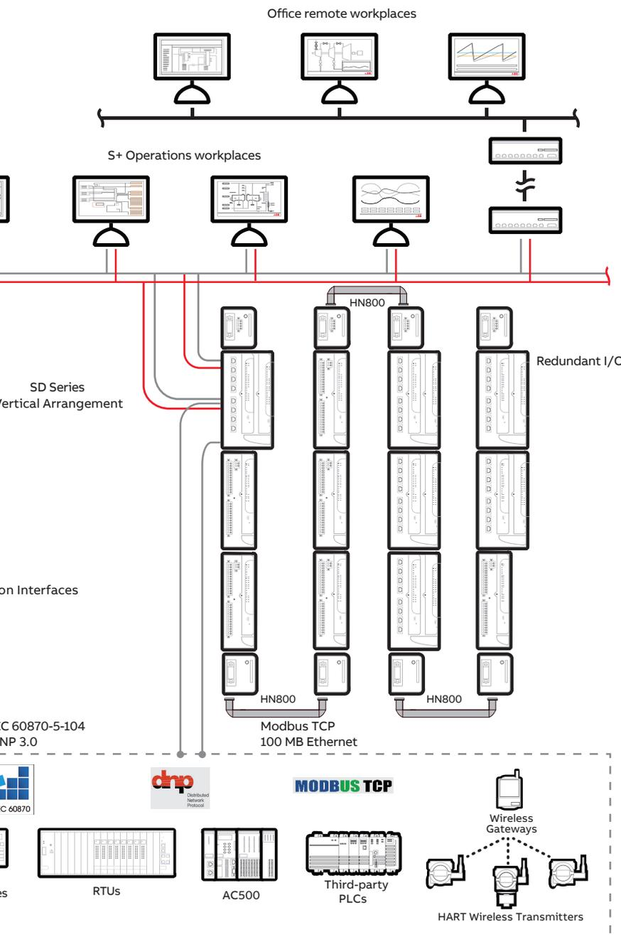
The SD Series features modular DIN rail packaging, a flexible, high-performance Fast Ethernet-based plant network, and intelligent electrical and field device integration via PROFIBUS, HART, IEC61850, IEC 60870-5-104, DNP 3.0 and Modbus TCP communication protocols. The SD Series also protects investments made in previous rack controllers and I/O, while delivering higher performance, reliability and capacity.
