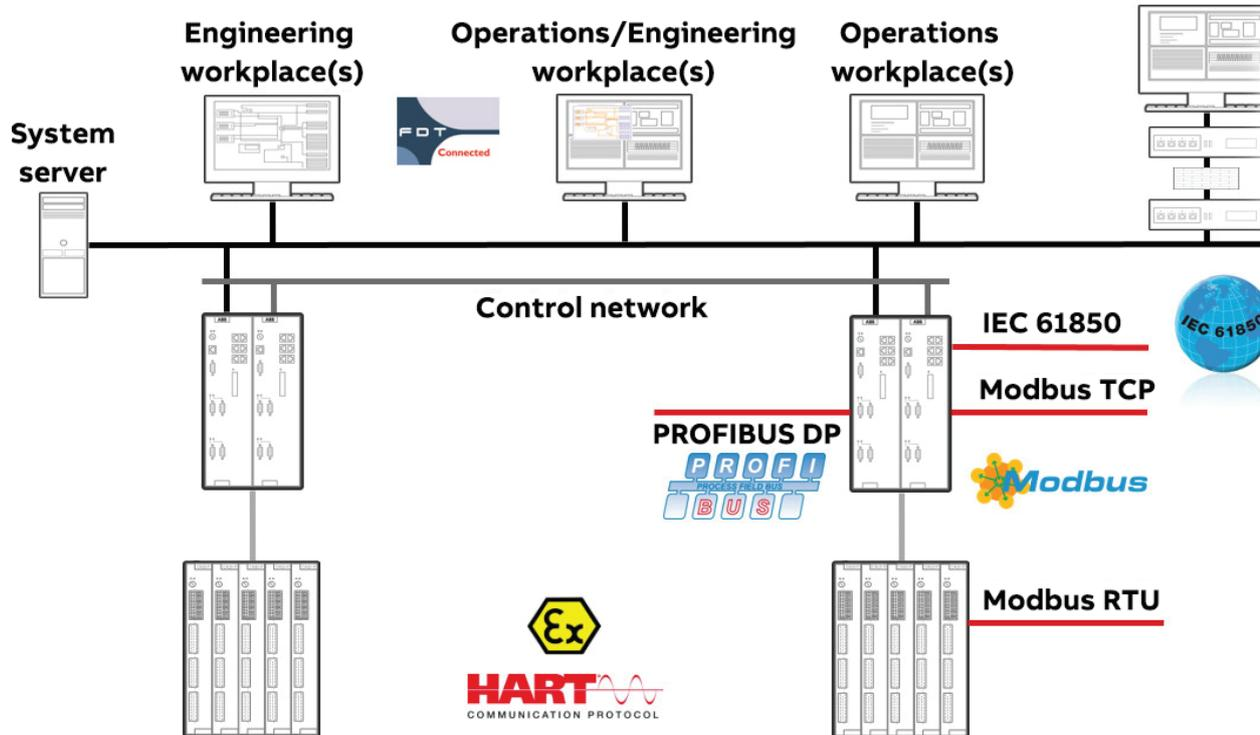
Symphony Plus MR Series (Melody Rack) controllers, communication interfaces and I/O modules meet the most challenging requirements. Thanks to their modular design, they can be easily adapted for a wide variety of plant types and sizes.
