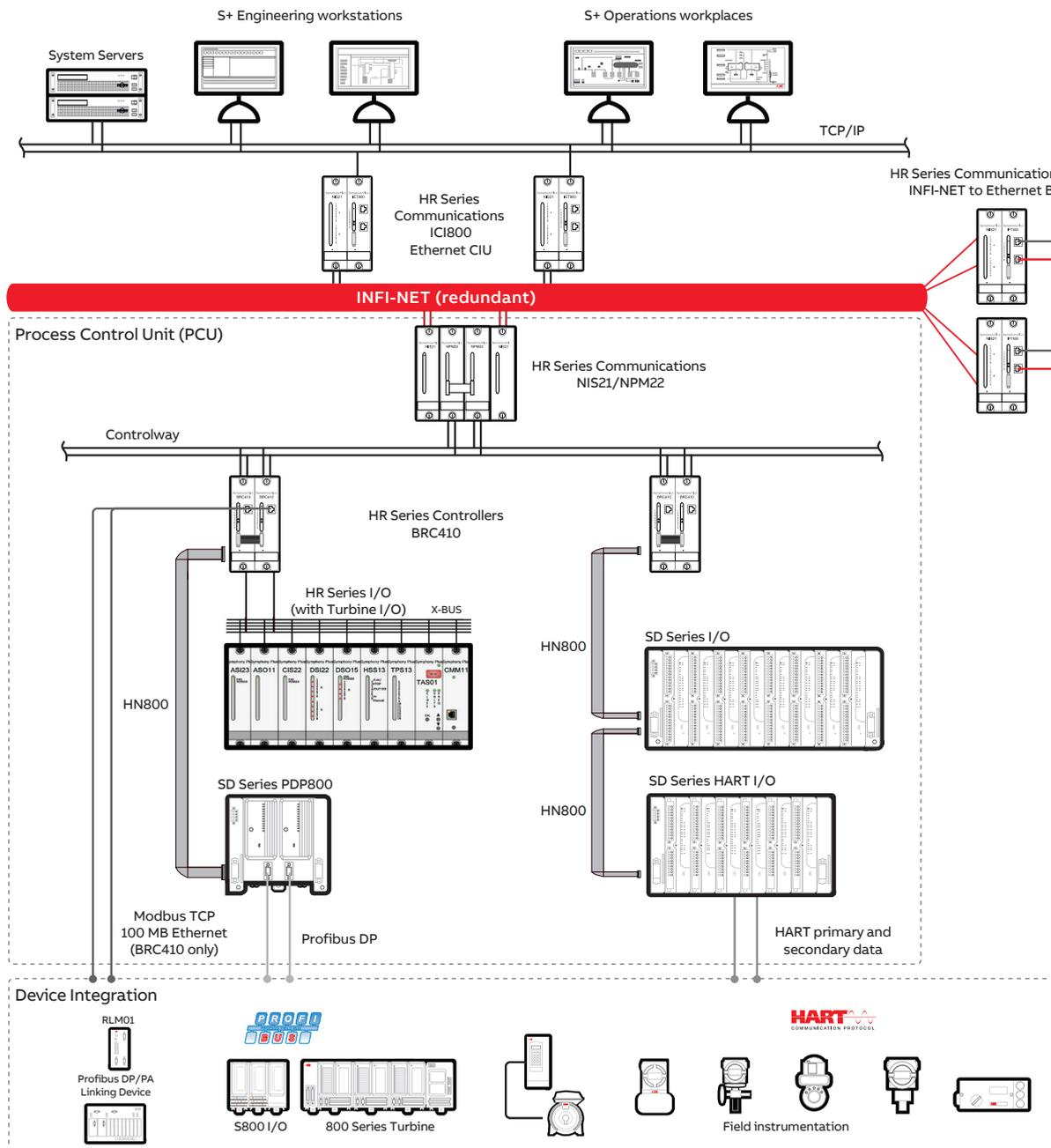
HR Series control-based systems feature scalable, high performance controllers, a comprehensive set of I/O options, fast, secure and redundant communication, an efficient easy-to-use engineering tool and a state-of-the-art HMI workplace.
