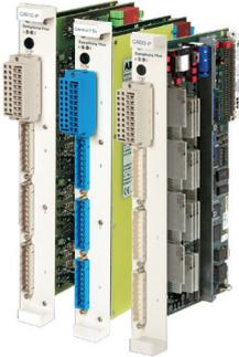
The inputs and outputs of the peripheral modules are connected to the signal lines with termination units. A Symphony Plus MR Series peripheral module has up to four front panel connection units. Signal lines can be assigned to 16 terminals (1 ... 16) for each termination unit.
