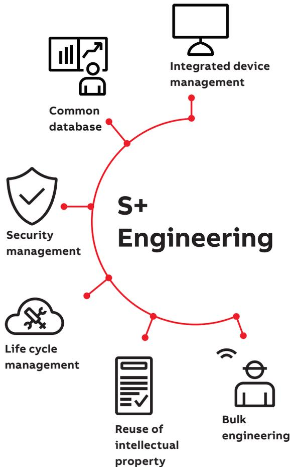
S+ Engineering is the configuration engineering tool used to engineer Symphony Plus systems based on SD Series, HR Series and SCADA architectures.
