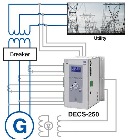
Figure 1 - DECS-250 Connection Diagram for a Typical Application
