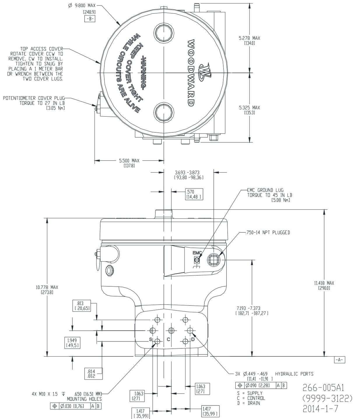
Figure 2-3a. Installation Drawing
