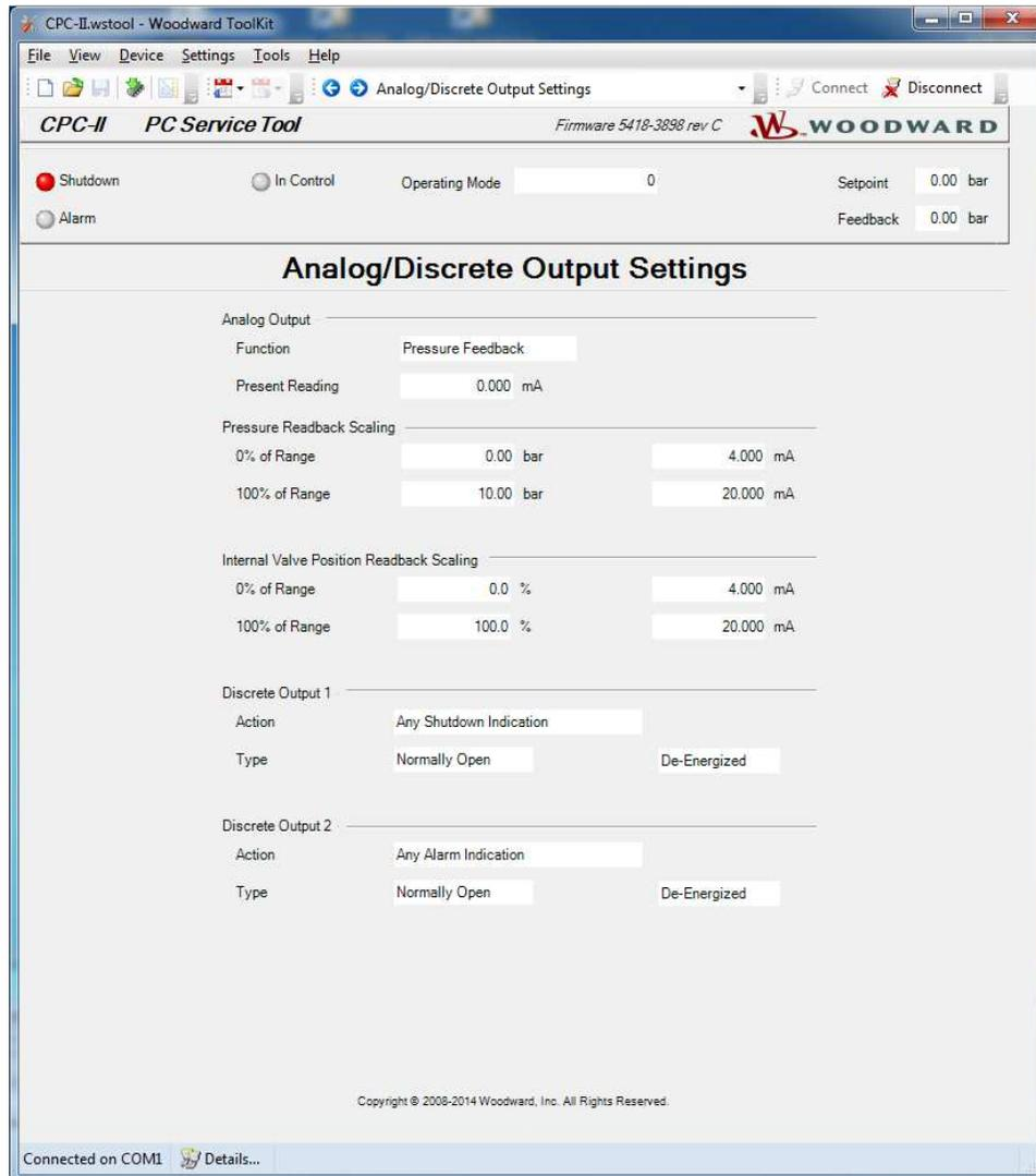
Figure 5-9. PC Service Tool Analog/Discrete Output Settings
