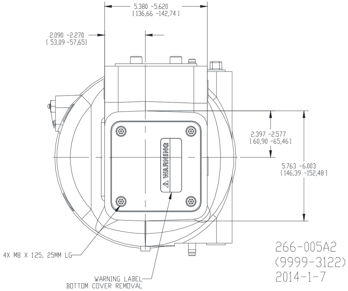
Figure 2-3b. Installation Drawing
