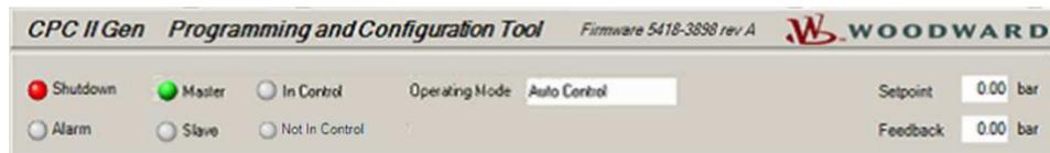
Figure 5-2. Common Header for Redundant Units (showing Master/Slave Status)
