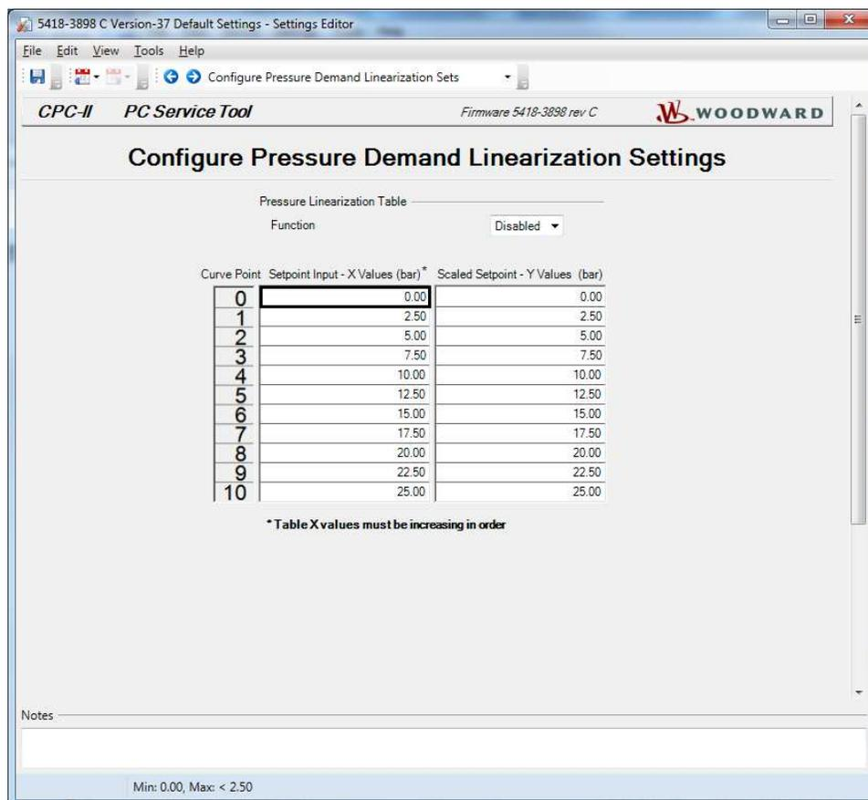
Figure 6-9. PC Service Tool Pressure Demand Linearization Configuration
