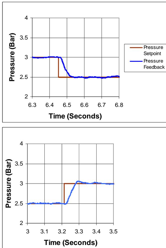
Figure 2-1. CPC-II Small Signal Step Response (Typical)
