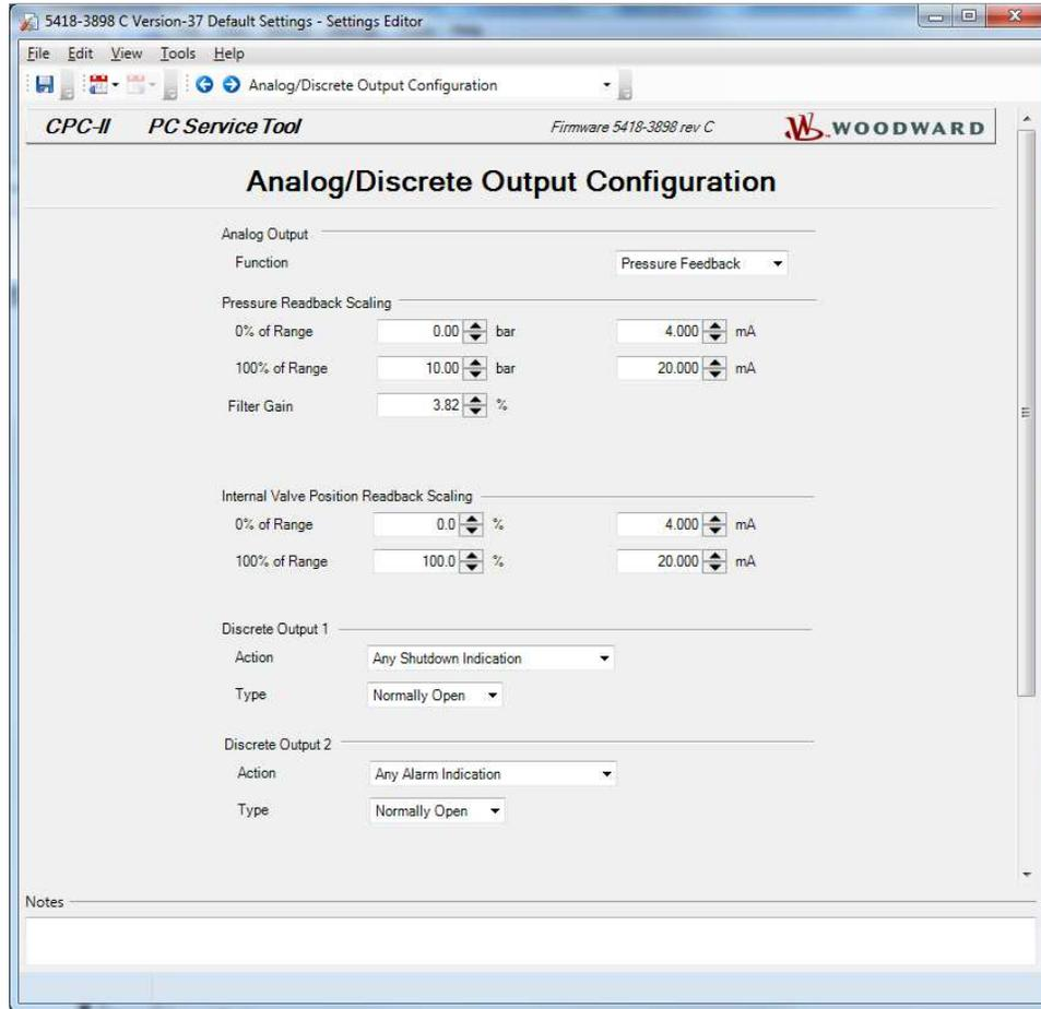
Figure 6-8. PC Service Tool Analog/Discrete Output Configuration
