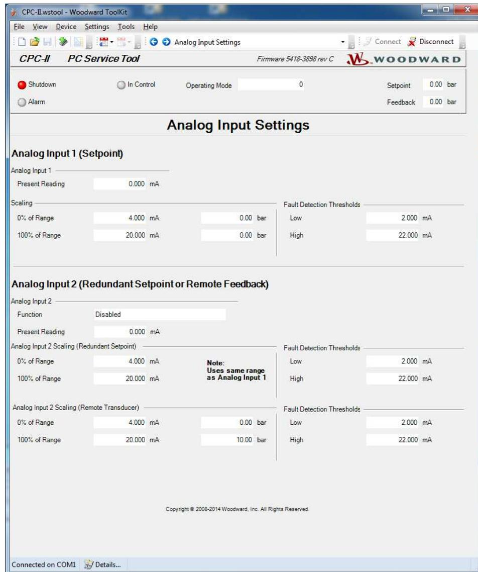
Figure 5-8. PC Service Tool Analog Input Settings
