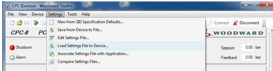
Figure 6-3. Loading the Settings File to the Device
