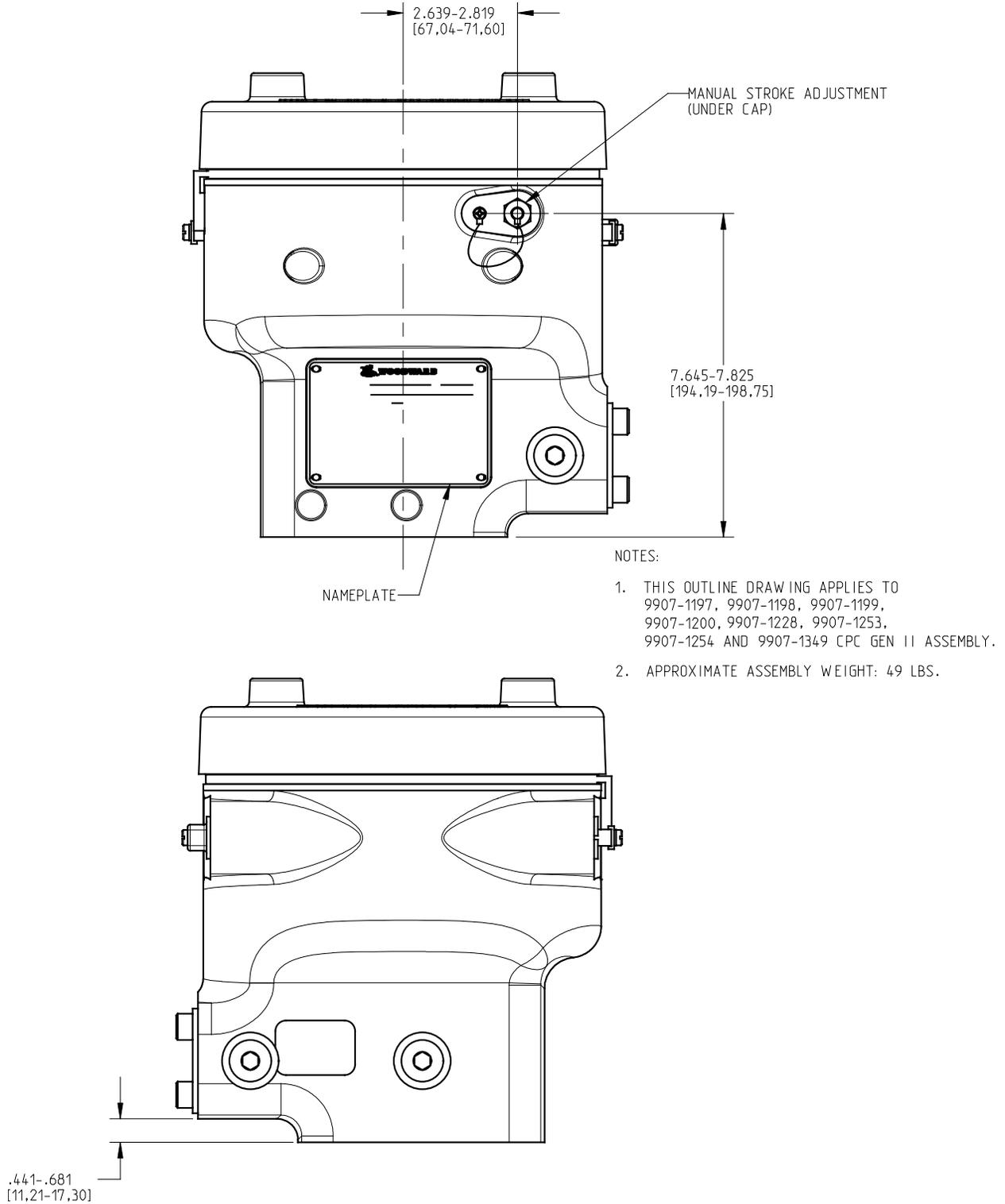
Figure 2-3c. Installation Drawing
