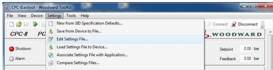
Figure 6-2. Loading the Settings File to the Device
