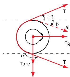
Horizontal measuring load cells
