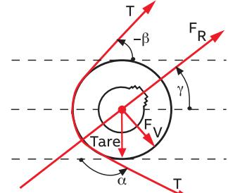
Diagonal measuring load cells
