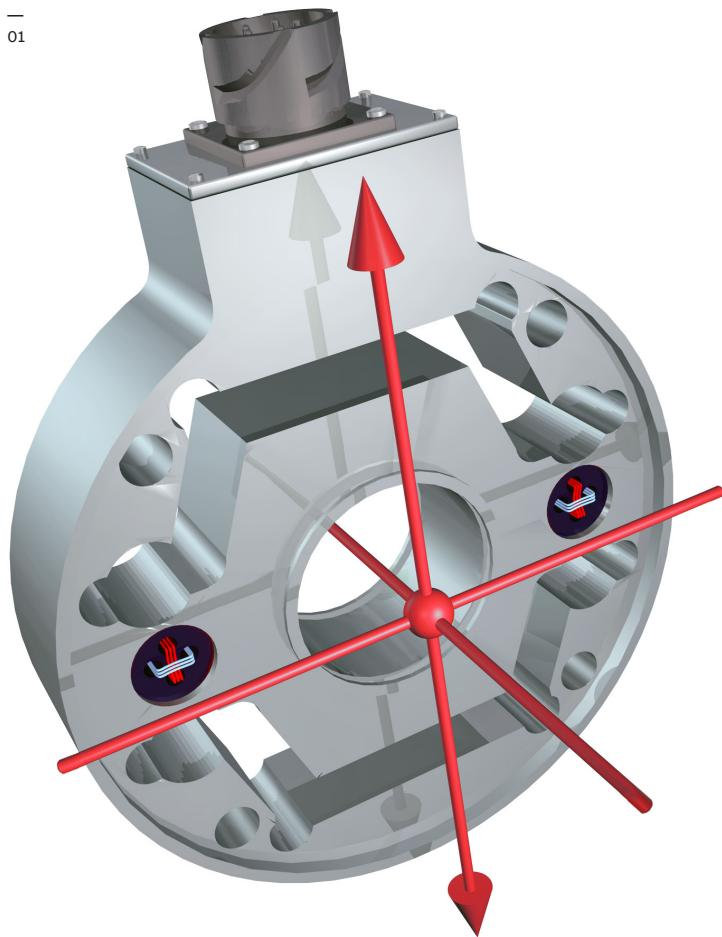
When horizontal, the measurement force ( $F_{R\text{tot}}$ ) is a function of just the tension in the web (T) and the deflection angles ( $\alpha$  and  $\beta$ ). Since the weight of the roll and bearings (Tare) is not sensed, the load cells can be sized to measure low tension levels even on a comparatively heavy roll. However, the perpendicular force ( $F_{V\text{tot}}$ ) – which does include Tare – should not exceed the overload rating.
