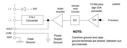
Accuracy is within " 0.5% maximum, " .2% typical over the entire span of the reading at 25C. This means accuracy is within 50mV on the 10 volt range, 5mV on the 5 volt range, and  $100\mu\text{A}$  on the 4 to 20 mA range. The blocks automatically calibrate all internal A/DandD/Acircuits periodically during normal operation.
