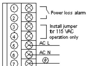
NOTE: A normally closed relay contact rated at 220 Vac, 6 A / 30 Vdc, 5 A is available on terminals 1 and 2 of the power terminal strip. This contact set may be used to signal input power OFF.
