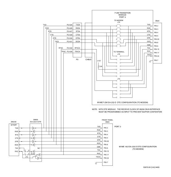
Figure 2-3. MVME162 EIA-232-D Connection Diagram, MVME712M (Sheet 3 of 6)
