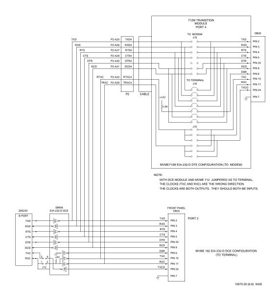
Figure 2-3. MVME162 EIA-232-D Connection Diagram, MVME712M (Sheet 6 of 6)
