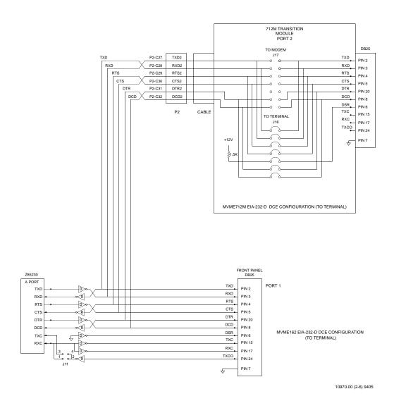
Figure 2-3. MVME162 EIA-232-D Connection Diagram, MVME712M (Sheet 2 of 6)
