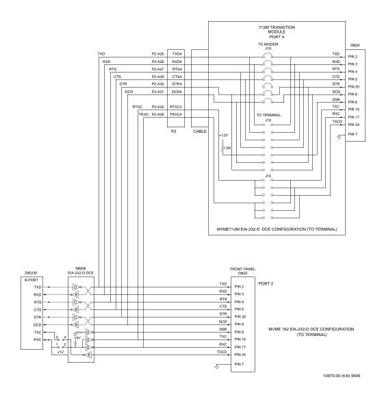
Figure 2-3. MVME162 EIA-232-D Connection Diagram, MVME712M (Sheet 4 of 6)
