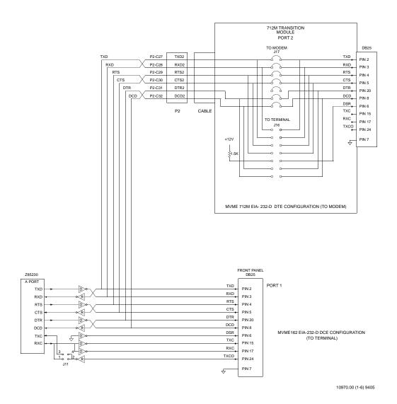
Figure 2-3. MVME162 EIA-232-D Connection Diagram, MVME712M (Sheet 1 of 6)
