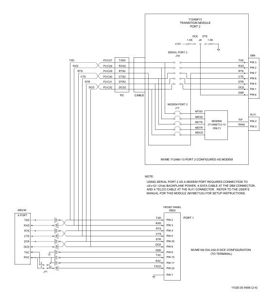
Figure 2-5. MVME162 EIA-232-D Connection Diagram, MVME712A/AM/-12/-13
