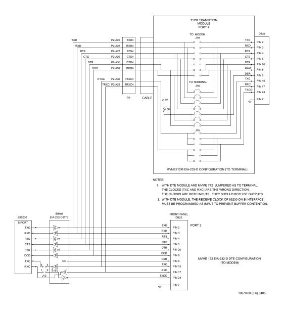
Figure 2-3. MVME162 EIA-232-D Connection Diagram, MVME712M (Sheet 5 of 6)
